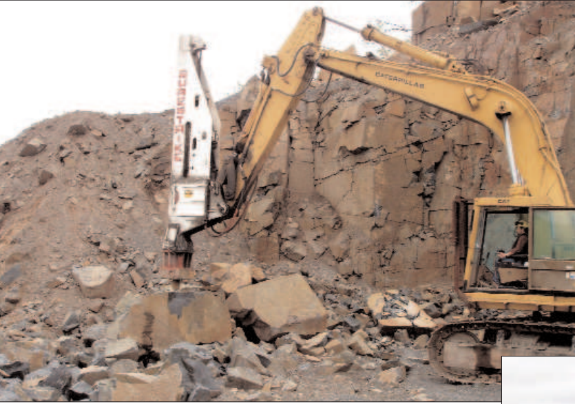
Easily mounted to a standard excavator, the Surestrike is a mechanical-impact hammer.
